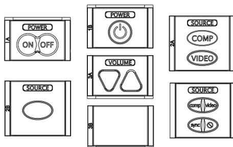
⊗ If the device you are controlling has discrete power buttons, use the ON/OFF combination, otherwise, use the toggling power
