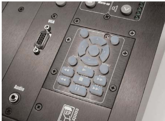
SP3-TCM+ mounted in a Large Chassis SmartPanel (SP2-CHAS)
