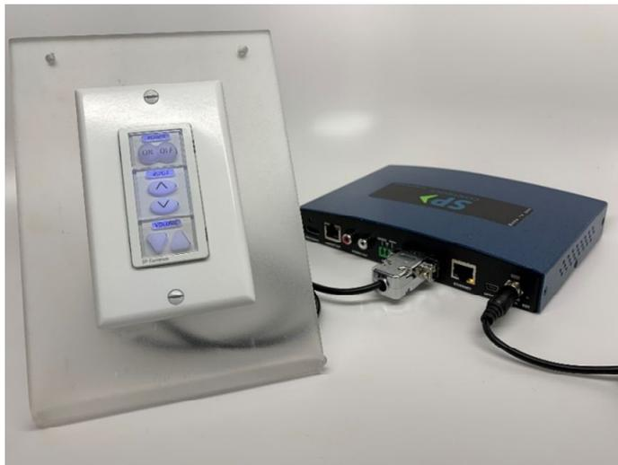
**HDBaseT POE & RS232** The PXE-KIT5200 provides an HDBaseT port for the transmission of 4K uncompressed audio and video to the projector. This product also offers PoE (PSE) power down the same cable to power the HDBaseT receiver. This means that a receiver can be mounted next to the project without the need of an additional power connection.
